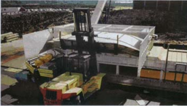
Waste Material Recycler RE-AS 3.200 x 6.700 for the resizing of rejected boards.
