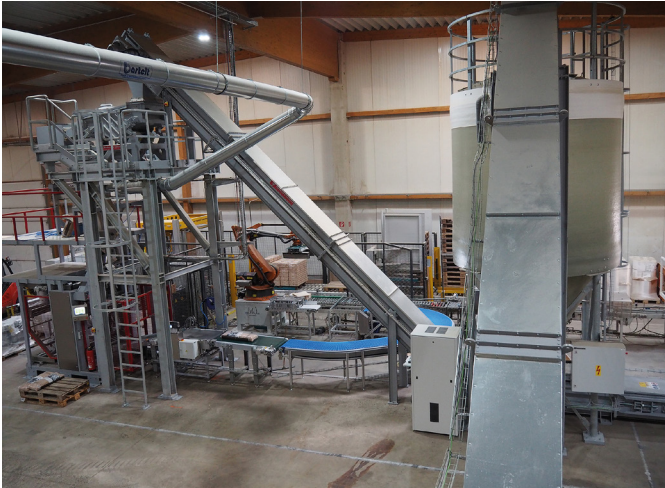
Rudnick & Enners also delivered a bagging machine which is connected to the exiting briquetting machine
