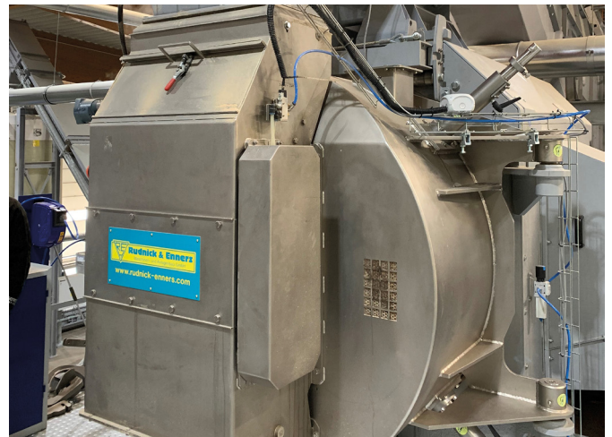
The Rudnick & Enners pellet press in use at Holz-Henkel is designed for an output of 5.5 t/h
