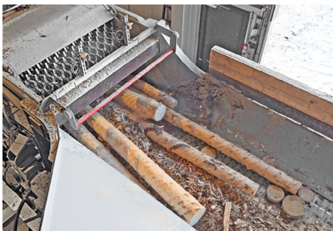
With its 200-kW motor, the shredder is also designed for shredding broken or pulp wood
