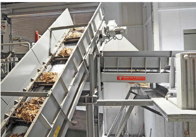
Robust step conveyors transport the bark to the shredder. Cuttings are fed in from the right
