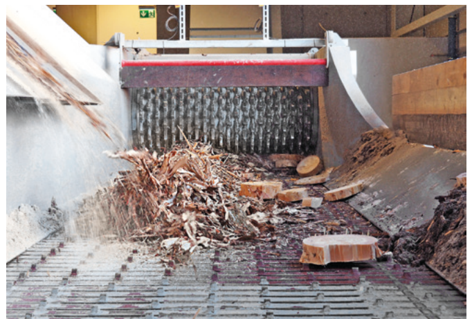
Rudnick & Enners GSA 1.600 shredder with a retractable counter-blade
