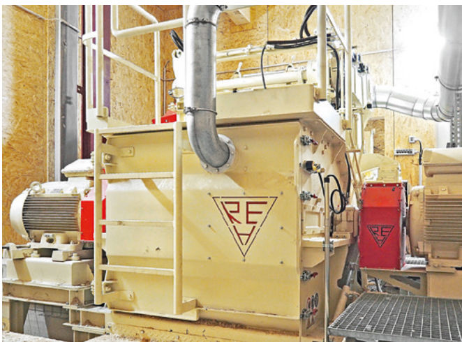
The Rudnick & Enners Twin Chipper is the heart of the wood waste disposal system in use at Westerwälder Holzwerke's sawmill for large-diameter logs
