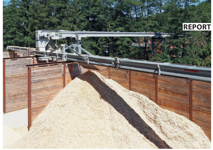
Two tubular belt conveyors transport sawdust and wood chips separately to the new residual wood bins at the edge of the premises.
