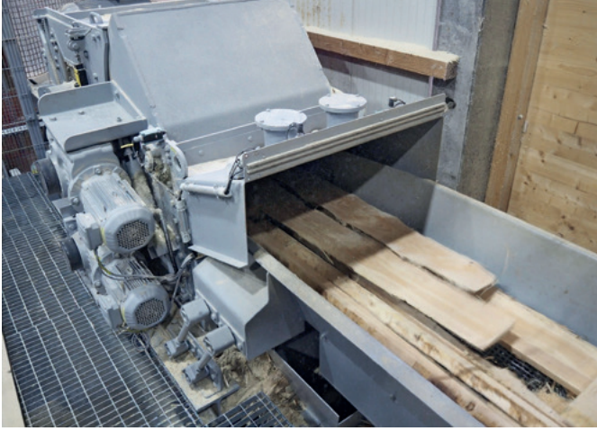
Rudnick & Enners delivered a TH 300/700/3 drum chipper with 90 kW drive power to Sägewerk Kolb
