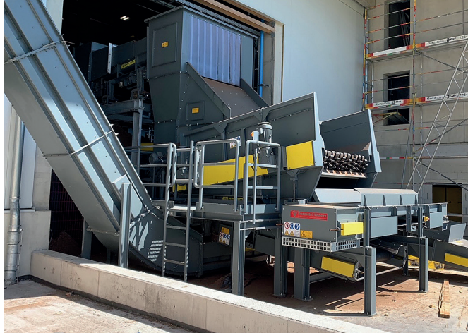
The RE RMV 1600 bark mill with the R&E star screen is used to sort out oversized grains
