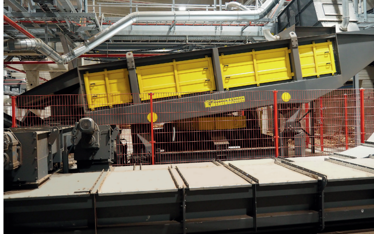
Rudnick & Enners's rotating screen for separating the wood waste
